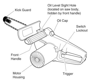
Figure 2 - Electric Chain Saw
